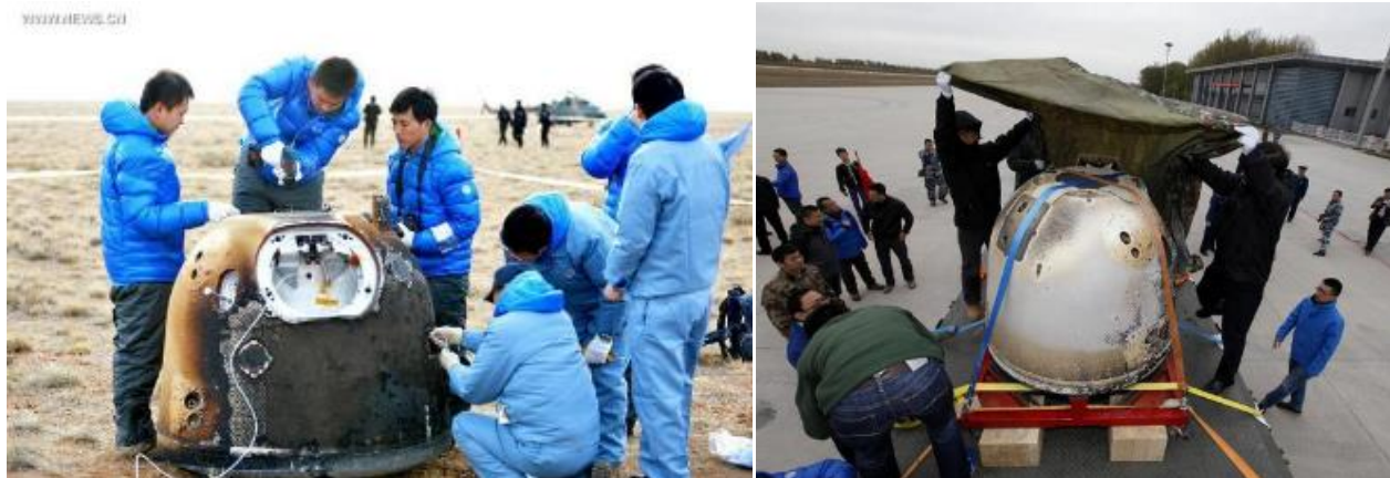
Figure 2.13. Left: the Chang'E-5-T1 return capsule during its recovery by the ground crews in Inner Mongolia on 31th October. Right: the recovery crew during the transportation at Beijing. The cradle is the support under the capsule. Credit: CNSA.
