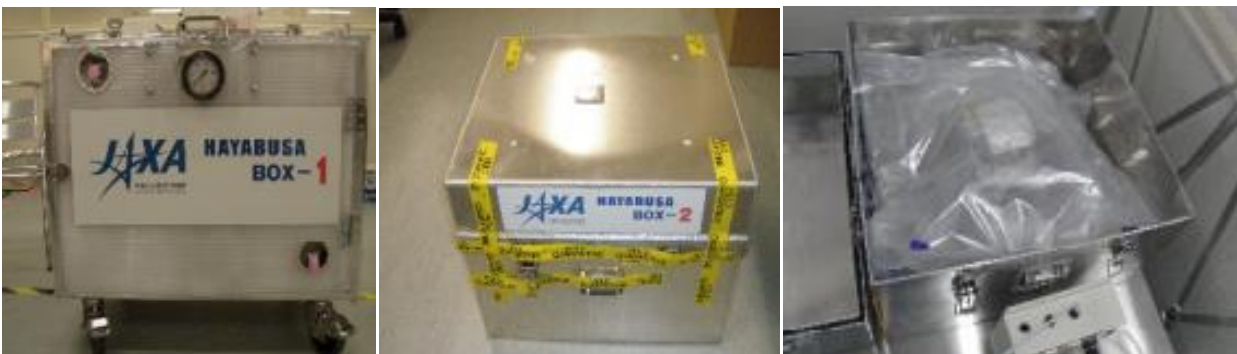
Figure 2.10. Left and centre: the two transportation boxes used for the Hayabusa 1 mission. The N 2 entrance and temperature sensor are placed externally. Right: the transportation box internal
