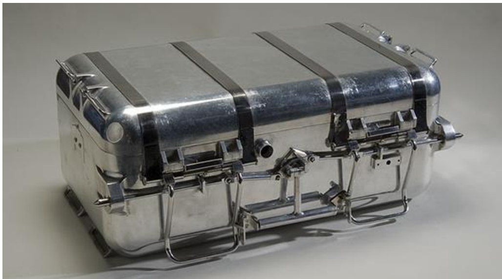
Figure 2.3. Apollo Lunar Sample Return Container (ALSRC). This container served on both the Apollo 12 and 16 missions (NASA photo S72-37196).
