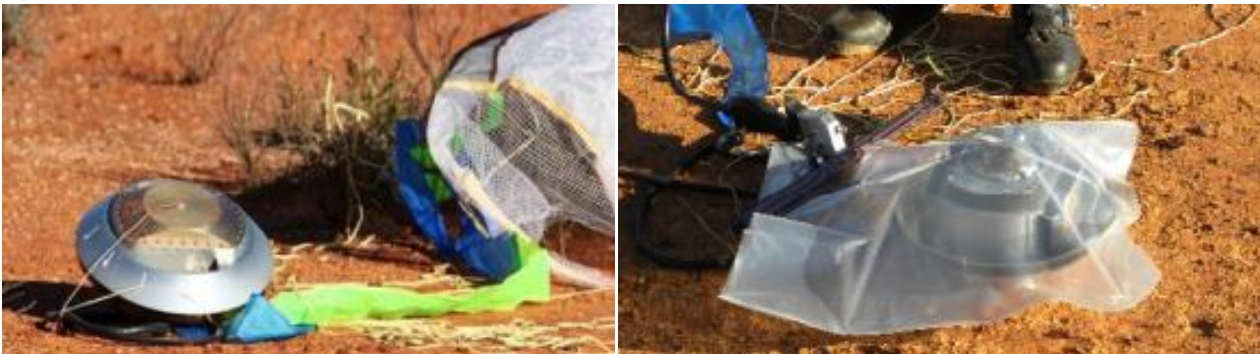
Figure 2.9. Left: Hayabusa 1 capsule returned. Right: the capsule packaging performed by the recovery team into a temporary plastic bag (from JAXA Report for Hayabusa 2, May 2014).
