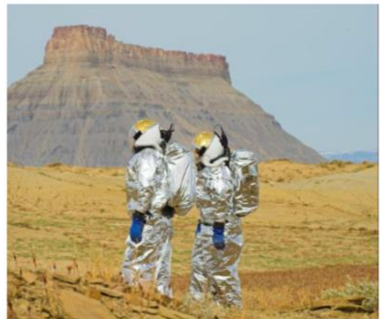
Fig.1: Mylar-foil shielded spacesuit simulators for tracking the contamination vectors during the AustroMars mission.
